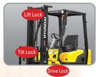
**OPSS (Operator Presence Sensing System)** Control of mast tilting, lifting and lowering is not possible through operation of the appropriate control when the operator is not in the normal position.(Option)
