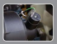
**Electrically monitored** air filter Air cleaner sensor alerts the operator of a restricted air filter and allows
